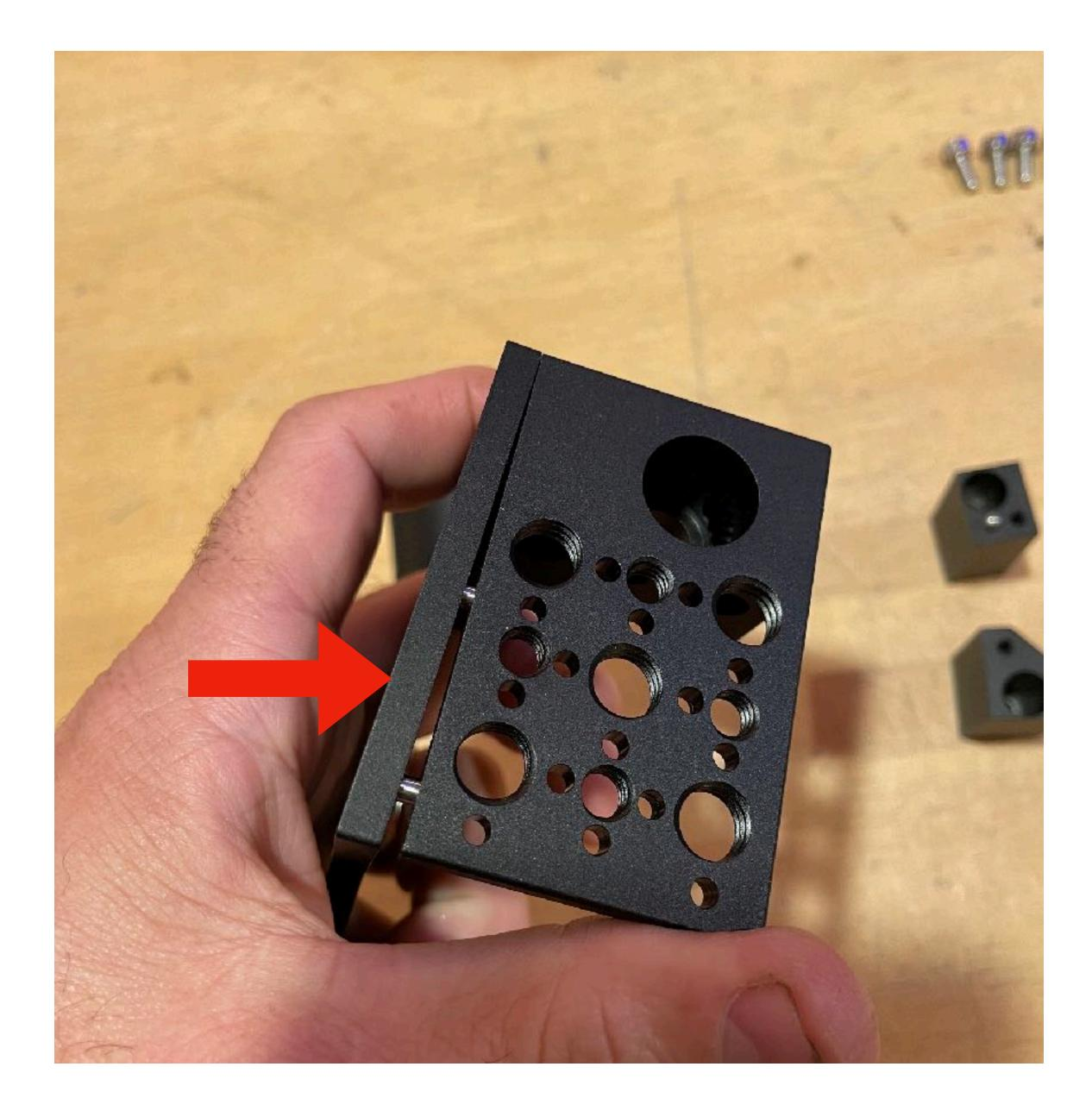
Using 2x M4x10mm screws attach the top block to the faceplate. DO NOT tighten these screws yet, leave them a little loose. If your cage is prebuilt then loosen these screws slightly at this point
