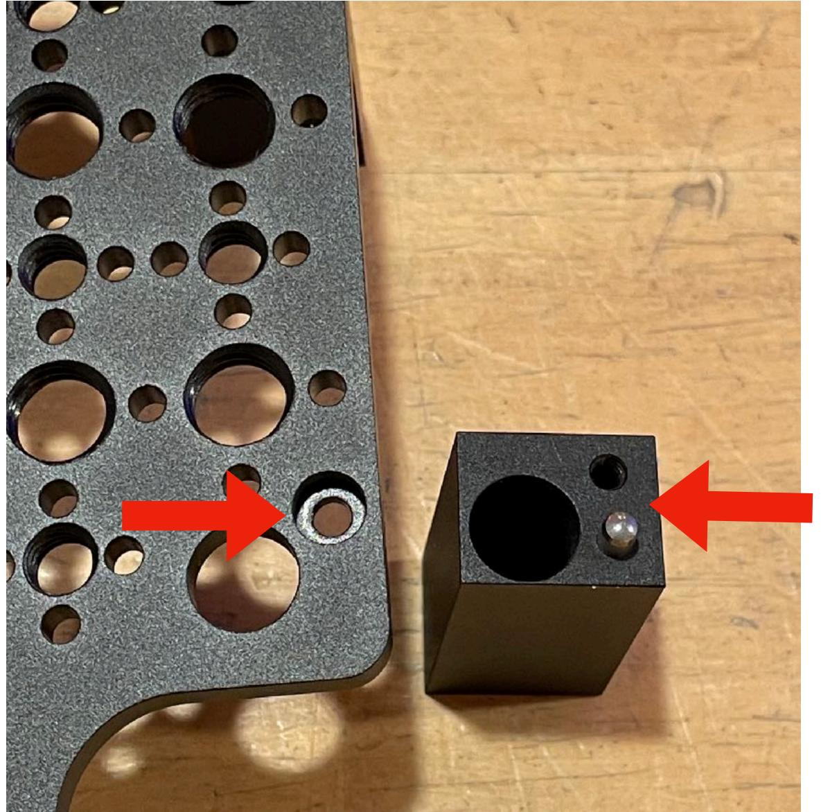
Next take the triangle stand off and align the dowel pin with the hole at the back of the faceplate as shown. Use 1x M3x10mm (the smallest of the bolts) to attach this to the faceplate. **DO NOT tighten yet. If your** cage is prebuilt please loosen this bolt now
